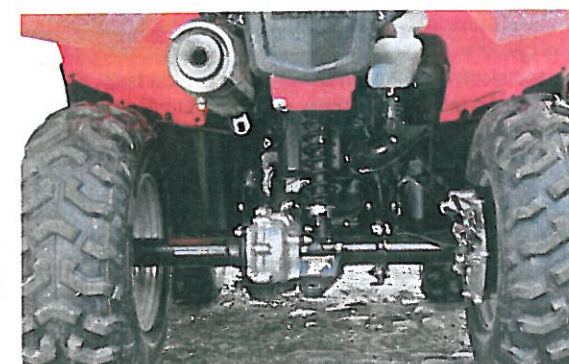
A single gas strut rear suspension is as simple as you can get, but the drum brake is now somewhat dated when compared to the others
